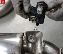
C) Rotate Scorpion valve so its in the same position as the O.E electronic valve motor.
